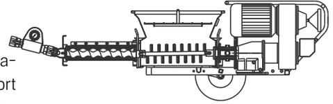
**Earth-moist clay plaster mortars** are mixed in batches and transported to the area to be plastered by robust mortar pumps ('open systems').
